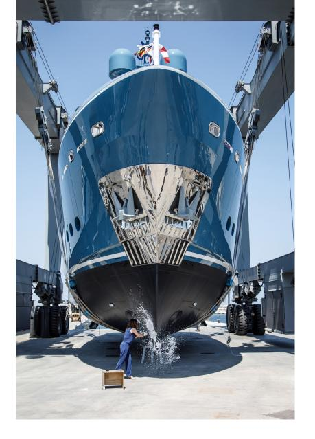
The project, customized according to his Owner precise requests, is designed to sail for long periods at the highest latitudes therefore Alexa features enhanced scantlings in the hull and rudders to cope with icy conditions. The Upper deck stern terrace will be built in steel instead of aluminium. All floors are heated and it is possible to close the cockpit to allow guests to enjoy the landscape even when the outside temperature is very low.
